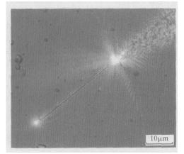
Fig. 4 Optical micrograph of launching 633nm light into a ZnO nanowire by means of a silica nanotaper
