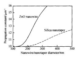
Fig. 3 Calculated propagation constants of a ZnO nanowire and a silica nanotaper at 633nm
