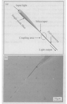
Fig. 2 Schematic diagram (a) and optical micrograph (b) of the evanescent coupling approach to launching light into a single nanowire
