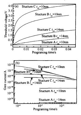
Fig. 5 Threshold voltage (a) and gate current (b) during programming processes Tunneling oxide thickness  $t_{ox} = 10$ ,14nm
