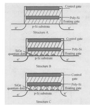
Fig. 1 Schematic structure of conventional full F-N memory cell (A) and the two proposed enhanced F-N tunneling memory cells (B and C)
