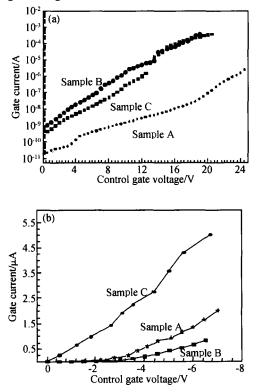
Fig. 8 Experimental results of gate current during programming (a) and erasing (b) for three structures
