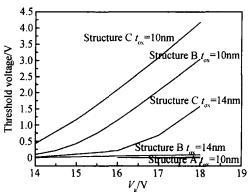
Fig. 7 Threshold voltage dependence on control gate voltage for the three structures Tunneling oxide thickness  $t_{ox} = 10$ ,14nm
