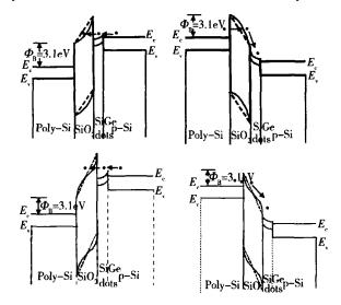
Fig. 4 Energy band diagrams of sturcture B (top) and C(bottom) Left for programming; right for erasing
