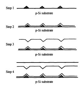
Fig. 2 Fabrication process of poly-Si floating gate with self aligned tips Step 1:self-assembled Si Ge dots; Step 2:Si films epitaxy; Step 3:oxidation; Step 4:poly-Si deposition
