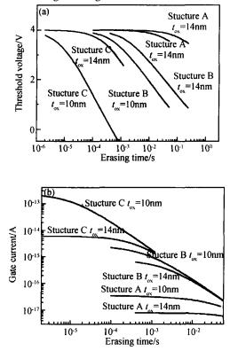
Fig. 6 Threshold voltage (a) and gate current (b) during erasing Tunneling oxide thickness  $t_{ox} = 10$ ,14nm
