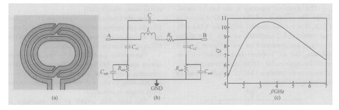
Fig. 7 (a) Microphotograph of the on-chip spiral inductor; (b) Model of the inductor; (c) Q-curve of the inductor
