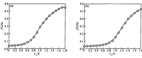
Fig. 13 Measured tuning characteristics of the VCO (a)  $V_{t1} = 0.8V$ ; (b)  $V_{t1} = 1V$
