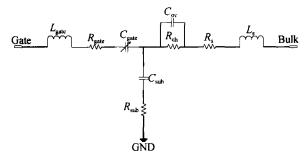
Fig. 9 Equivalent circuit of a MOS varactor
