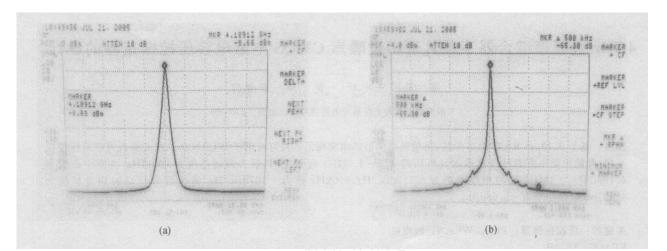
Fig. 14 Spectrum of the 4. 1887 GHz output signal (a) Measured output power (SPAN 10M Hz); (b) Measured phase noise (SPAN 2M Hz; VBW 1k Hz; RBW 10k Hz; Centre 4. 189 GHz; frequency off set 500k Hz)
