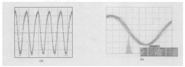
Fig. 15 (a) Measured PLL output waveform (200ps/div) in time domain at 4. 22 GHz; (b) Jitter of the output
