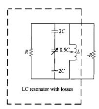
Fig. 6 Equivalent circuit of the oscillator
