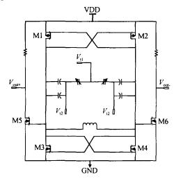
Fig. 5 Circuit schematic of the VCO
