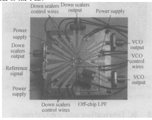
Fig. 12 Photograph of the test PCB
