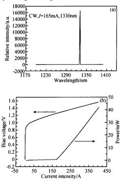
Fig. 4 (a) Laser spectrum of a 3mm-cavity-length InAs QD laser operating in CW mode measured at room temperature; (b) Light output characteristics and bias voltage versus current of the lasers
