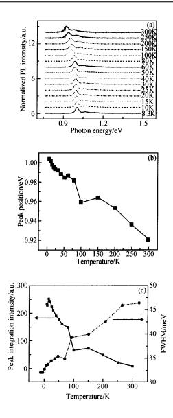
Fig. 3 Temperature dependent PL spectra of sample 1C with an excitation power of 16mW (a) Normalized intensity; (b) Peak position; (c) Integration intensity and FWHM of the low energy peak
