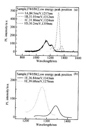
Fig. 2 PL spectra of samples 1A ,1B ,1C ,and 1D (a) , and 1E and 1F (b) at room temperature with an excitation power of 16mW
