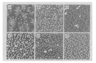
Fig. 1 AFM images (a) ~ (f) of InAs QDs of samples 1A ~ 1F grown by MBE on GaAs (001) substrate (1 $\mu$ m ×1 $\mu$ m area for all images)
