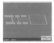
Fig. 2 SEM photograph of inductor sample with CoZrO thin-film
