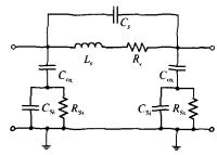
Fig. 3 Equivalent circuit of air-core on-chip spiral inductor
