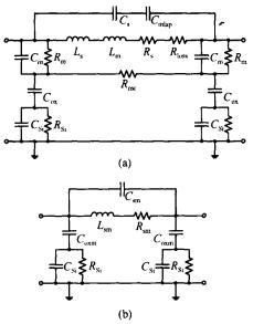
Fig. 4 Equivalent circuit of on-chip inductor with under-spiral magnetic thin-film (a) Modified two-port circuit with magnetic film added; (b) Simplified circuit of inductor with ferrite thin-film
