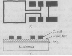
Fig. 1 Structure of RF integrated inductor with ferrite thin-film (a) Overhead view of the spiral coil; (b) Cross-sectional view
