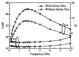
Fig. 5 Comparisons of L and Q between sample with ferrite film and reference inductor without ferrite film
