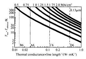
Fig. 8 Temperature rises on the globe line (in the 6th metal layer for 0.  $13\mu$ m generation) in the case without metal lines in the lower metal layers for different dielectric configuration (A) Homogeneously inserted aerogel; (B) Embedded aerogel; (C) Homogeneously inserted polymer low- k material; (D) Dense SiO<sub>2</sub>
