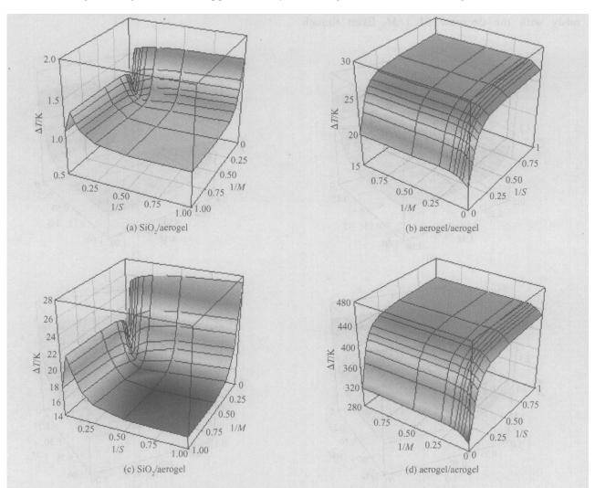
perature rises for the Ield/Iald dielectric configuration aerogel/aerogel are approximately  $k_{SiO_2}/$   $k_{aerogel}$  times higher than those in the  $SiO_2/$  aerogel or  $SiO_2/SiO_2$  configurations.
