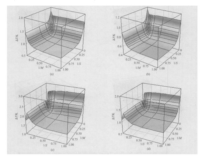
Fig. 5 Temperature rises from the substrate to the top metal line for dielectric configuration of  $SiO_2/aero-gel (Ield/Iald)$  for Al and Cu metallization with  $J = 0.5 MA/cm^2$  (a) Al, current through the top metal line; (b) Cu, current through the top metal line; (c) Al, current through all metal lines; (d) Cu, current through all metal lines
