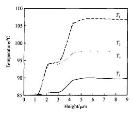
Fig. 4 Temperature distribution of the three-metallayer Cu interconnect structure at x = 0 (refer to Fig. 1) for various technologies
