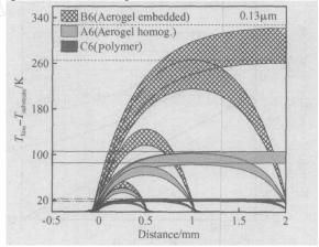
Fig. 9 Temperature distribution along the global lines above unoccupied lower metal layers between function blocks of 0. 5 ,1 ,2 , and 4mm distance for 0.  $5MA/cm^2$
