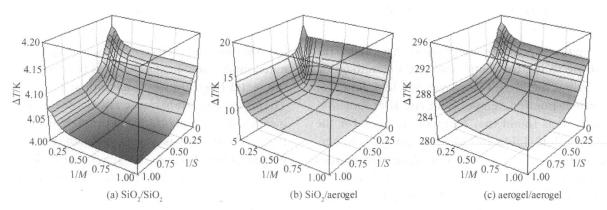
Fig. 7 Temperature rises from the substrate to the top metal line of Cu metallization for various kinds of dielectric employment for Ield/Iald Here the current propagates only through the top metal line with  $J = 2MA/cm^2$ .
