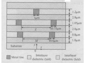
Fig. 1 Schematic cross section of the simulated interconnection structure
