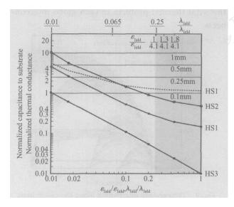
Fig. 11 Dependence of normalized thermal conductance (solid line) and capacitance (dashed line) on the ratio of thermal conductivity and dielectric constants for different types of dummy heat sinks, respectively The quantities are normalized to the corresponding values of a 100 $\mu$ m long uncooled interconnect of level M6 (0. 13 $\mu$ m). Horizontal lines refer to uncooled interconnects of different lengths.
