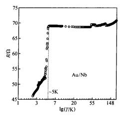
Fig. 2 *R*-*T* curve of Au/Nb
