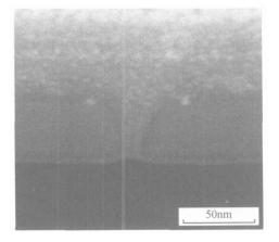
Fig. 1 Cross section of hole filled by sputtering
