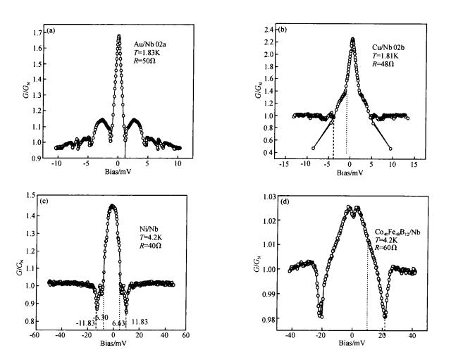
Fig. 3 (a) Normalized GV curve of Au/Nb contact; (b) Normalized GV curve of Cu/Nb contact; (c) Normalized GV curve of Ni/Nb contact; (d) Normalized GV curve of Co<sub>40</sub> Fe<sub>48</sub>B<sub>12</sub>/Nb contact
