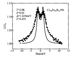
Fig. 4 Normalized GV curve of Co<sub>40</sub> Fe<sub>40</sub> B<sub>20</sub>/Nb contact by Nb tip method The straight line is the BTK fit. For thermal broadening of the spectrum, only the key feature of the gap structure is fitted by T = 2 K, = 1. 225 meV, Z = 0.03.
