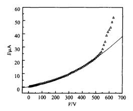
Fig. 2 Current versus applied voltage of cBN crystal shown in Fig. 3.
