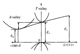
Fig. 4 Scheme of the energy band of cBN crystal At 300 K:  $E_g = 6.1 \sim 6.3 \text{ eV}$ ,  $E = 8.5 \sim 10 \text{ eV}$ ,  $E_L > 12 \text{ eV}$
