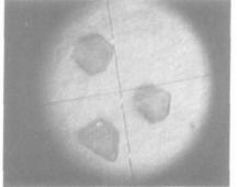
Fig. 1 Microscope photograph of cBN sample The cBN in top left corner was used in our experiment.  $S = 0.1427 \text{ mm}^2$ , L = 0.06 mm
