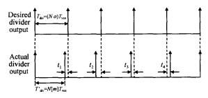
Fig. 3 Ideal and actual frequency divider output signal in the time domain
