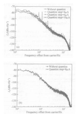
Fig. 9 (a) Spurs arise due to compensation current quantization; (b) Spurs becomes negligible when  $I_{cp}$  is increased to 1. 2mA with a 8µA quantization step
