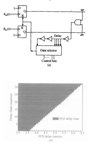
Fig. 10 (a) Delay programmable PFD; (b) Simulation results of the PFD delay time
