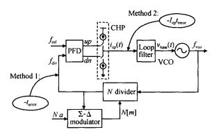
Fig. 2 Structure of the sigma-delta fractional-N frequency synthesizer
