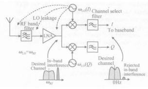
Fig. 1 Direct-conversion receiver
