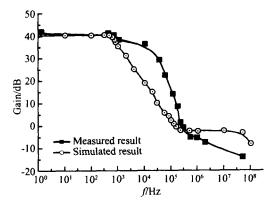
Fig. 5 Measured frequency response of the DM feedback-loop
