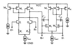
Fig. 3 DM feedback loop with Miller multiplier
