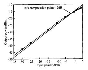
Fig. 6 Measured input 1dB compression point
