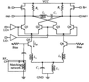
Fig. 2 Schematic of double balanced mixer
