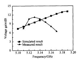
Fig. 7 Measured conversion voltage gain
