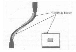
Fig. 2 Top view and cross section of S-bend VOA
