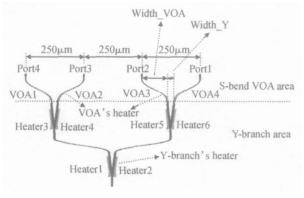
Fig. 1 Schematic of 1 ×4 DOS
