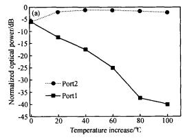
Fig. 3 Simulation of the output with heater 1 and heater 6 working at the same time
