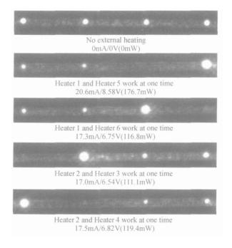
Fig. 4 Four different output states under certain driving power when the corresponding heaters work at the same time
