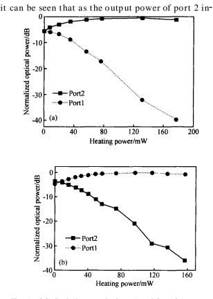
Fig. 5 (a) Optical power in Port 1 and Port 2 versus heating power with heater1 and heater6 working at the same time; (b) Optical power in Port 1 and Port 2 versus heating power with heater 1 and heater 5 working at the same time
