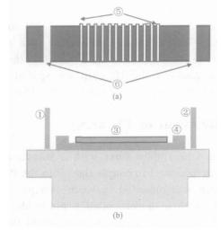
Fig. 2 Schematic of alignment for PD array and 1 ×12 ribbon fiber with MT connector (a) 1 ×12 ribbon fiber with MT connector; (b) Pin-holder and A-lignment pins; PD array; Protective base; Multi fibers; Alignment holes
