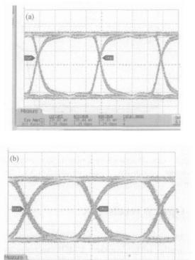
Fig. 4 Typical channel eye pattern for 23bit PBS (a) 1. 25 Gbit/s; (b) 2. 5 Gbit/s
