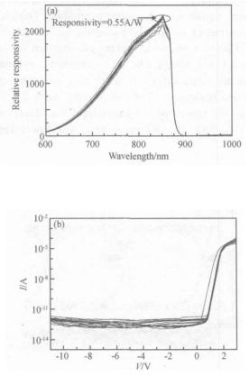
Fig. 1 Opto-electric characteristic of PD array (a) Relative responsivity versus wavelength; (b) *FV* curves
