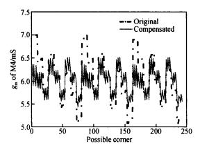
Fig. 5 Simulation results of the transconductance of M4 in all possible corners in compensated and un compensated circuits
