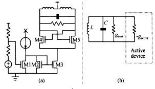
Fig. 1 Schematic (a) and equivalent circuit (b) of an LC oscillator  $% \left( {{\left[ {{L_{\rm{B}}} \right]} \right]_{\rm{B}}} \right)$
