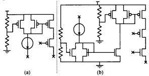
Fig. 3 Bias current compensation for pMOS (a) and CMOS (b) transistors
