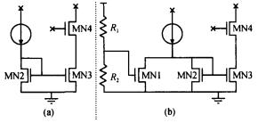
Fig. 2 Two bias current schemes for an nMOS transistor (a) Original one without compensation; (b) Improved one with compensation
