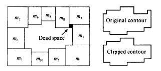
Fig. 2 Mark the dead space and clip the contour
