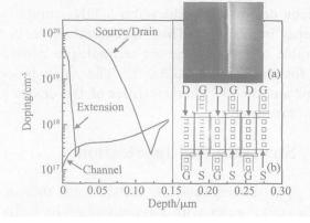
Fig. 2 Simulated doping profiles Insets are SEM image of 0.  $18\mu$ m gate line (a) and multi-finger gate structure (b).
