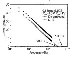
Fig. 4 Current gain versus frequency of  $0.18\mu$ m nMOSFET
