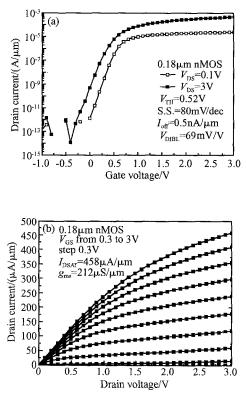
Fig. 3 DC characteristics of 0. 18µm RF nMOSFET (a) Transfer characteristics; (b) Output characteristics
