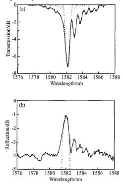
Fig. 4 Measurement and simulated results of transmission (a) and reflection (b) for TE mode of a Bragg grating
