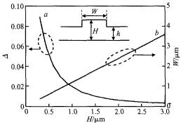
Fig. 1 Dependence of refractive index difference ( ) and waveguide width ( W) on substrate thickness ( H) for h/ H = 2/3
