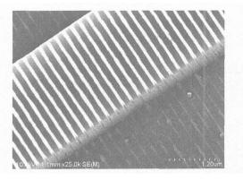
Fig. 3 Bragg grating on an SOI rib waveguide
