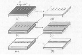
Fig. 2 Fabrication process of Bragg gratings on rib waveguides
