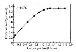
Fig. 6 Plot of oxidation rate versus the carrier gas flux
