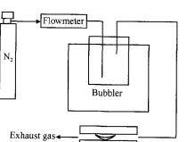
Furnace Fig. 1 Experimental setup for oxidation
