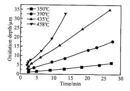
Fig. 4 Measured lateral oxidation depth versus time for mesa with PR at different temperatures
