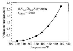
Fig. 5 Plot of oxidation rate versus temperature
