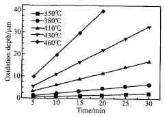
Fig. 2 Measured lateral oxidation depth versus time for the mesa with stripe at different temperatures
