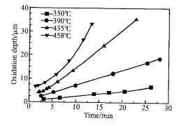
Fig. 3 Measured lateral oxidation depth versus time for mesa with RT at different temperatures
