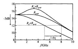
Fig. 4 Bandwidth extension by active inductor
