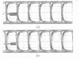
Fig. 10 Eye diagrams with optical signal input at  $-15dBm(23.3\mu A)$  (a) and  $-17dBm(15.8\mu A)$  (b)
