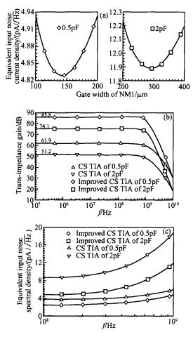
Fig. 6 Spectral simulation results (a) Equivalent input noise current density versus gate width of NM1; (b) Simulated frequency responses; (c) Equivalent input noise spectral density
