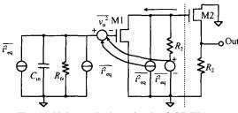
Fig. 5 Noise equivalent circuit of CS TIA
