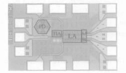
Fig. 8 Microphotograph of the front-end amplifier
