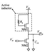
Fig. 3 Active inductor shunt peaking
