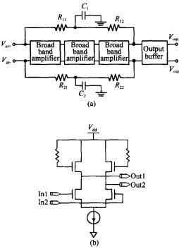
prove the bias stability and reduce the crosstalk among stages ,we adopt direct coupling between staFig. 7 (a) Limiting amplifier structure; (b) Broadband amplifier
