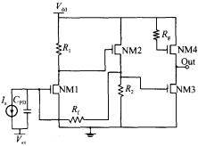
Fig. 2 Diagram of improved CS TIA
