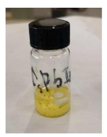
Figure S1. The photo of the  $CsPbI_3$  crystals obtained via antisolvent-assisted precipitation strategy.
