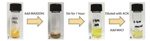
Fig. S1. (Color online) The solution preparation process and photographs of the samples.
