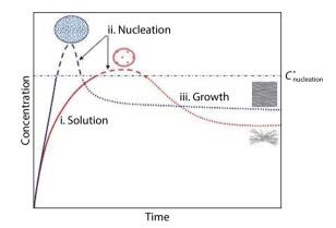
Fig. S3. (Color online) Lamer model to explain the nucleation and crystal growth in DMF/DMSO solution (red line) and MA(EtOH)/ACN solution (blue line). Solid line for solution stage; long dash line for nucleation stage; dot line for crystal growth stage.
