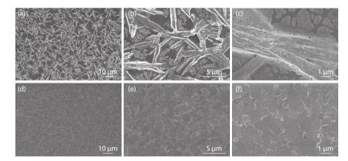
Fig. S4. (Color online) Top-view SEM images for perovskite films made from (a-c) DMF/DMSO solution, and (d-f) MA(EtOH)/ACN solution.
