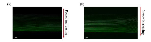
Figure 5. Confocal fluorescence microscope image of the  $1^{st}$  layer. (a) Fresh sample, (b) aged sample. The aging samples were placed in an environment with a relative humidity of 85% and 85 °C for 96 hours. The scale bar is 8  $\mu$ m.
