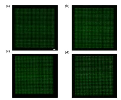
Figure 2. (a)-(d) Confocal fluorescence microscope images of dots written by a fs laser with a single pulse of precise energy in PC, PCC, PS, and PMMA, respectively. The excitation wavelength was 405 nm, and the scale bar was  $10 \mu m$ .
