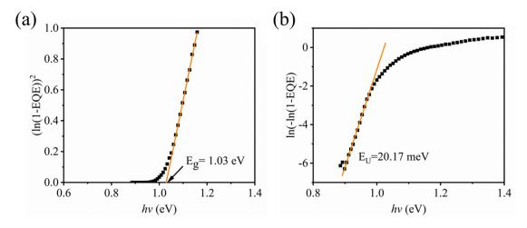
**Fig. S1.** (a) Band gap of the champion CISSe solar cell on FTO substrate. (b) Urbach energy of the champion CISSe solar cell on FTO substrate.
