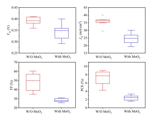
**Fig. S2.** The box-plots of the statistical device photovoltaic parameters of CISSe solar cells on FTO substrate without and with MoO<sub>3</sub>.
