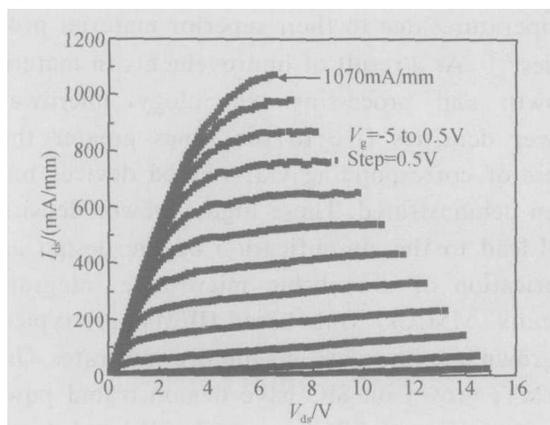
Fig. 5 Pulse measurement of  $80 \times 10 \mu\text{m}$  power device's  $I-V$  curves
