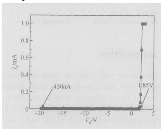
Fig. 4 Forward and reverse gate diode characteristics ( $W_g = 40 \mu\text{m}$ )
