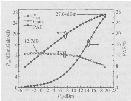
Fig. 7 Power performance of the 80  $\times$  10 $\mu\text{m}$  device ( $f = 8\text{GHz}$ ;  $V_{ds} = 10\text{V}$ )
