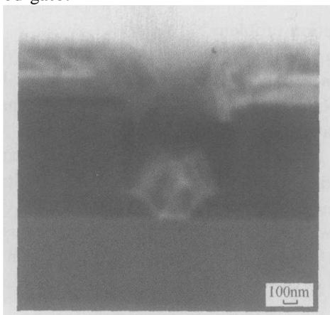
Fig. 2 SEM photo of  $0.25 \mu\text{m}$  T-shaped gate
