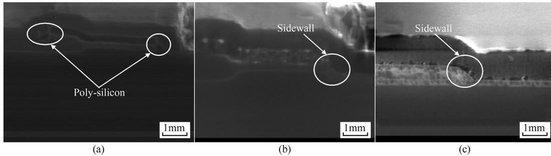
Fig.4 SEM pictures of HVpMOS device fabricated by different DGO processes (a) Normal DGO process without extra sidewall for HVpMOS; (b) Novel DGO process described as Fig. 2; (c) Improved DGO process based on that proposed in Fig. 2
