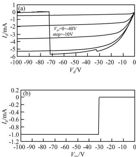
Fig. 3 (a)  $I_d$ - $V_d$  curves of HVpMOS; (b) Breakdown characteristics of 200nm thick gate oxide
