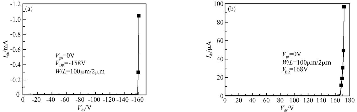
Fig.6 (a) Breakdown characteristics of HVpMOS; (b) Breakdown characteristics of HVnMOS
