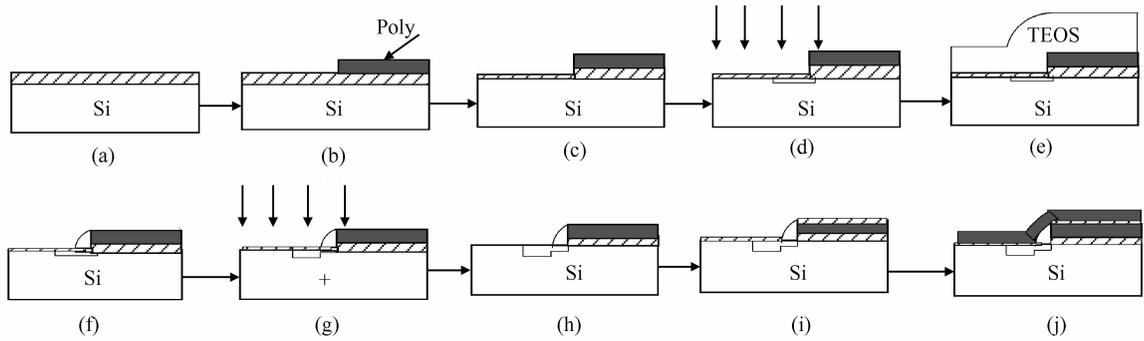
Fig. 2 Schematic of dual gate oxide process (a) 200nm thick gate oxide TEOS; (b) Poly-silicon etched; (c) Dry etch gate-oxide and 10~20nm retained; (d) p-implantation; (e) TEOS deposited; (f) Plasma etching TEOS and 10~20nm TEOS retained; (g) S/D implantation; (h) Wet etching  $\text{SiO}_2$  by 50 : 1 HF; (i) 15nm thin gate oxide; (j) Second poly-silicon
