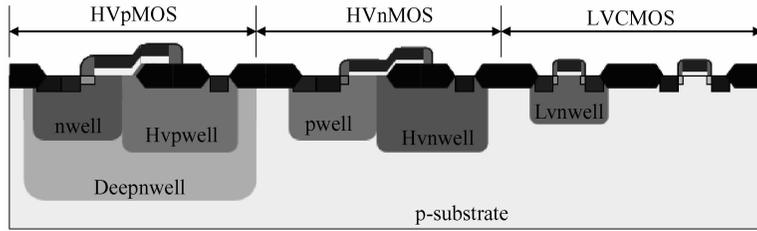
Fig. 1 Cross-sectional schematic of HVCMOS devices
