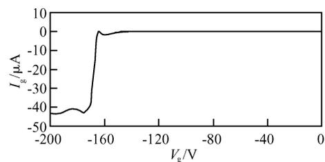
Fig.5 Breakdown characteristics of gate-source for HVpMOS device fabricated by the modified DGO process
