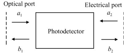
Fig.2 Schematic showing electrical waves and optical power flowing in and out of the photodetector
