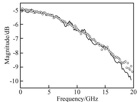
Fig.5 Magnitude of  $S_{21}$  before and after further calibration (solid line: before calibration; dotted line: after calibration)
