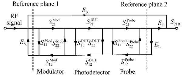
Fig.4 Flow graph of  $S_{21}$  measurement system
