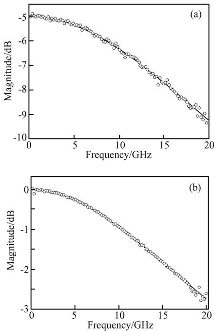
Fig. 6 Comparison between calculated and measured  $S$  parameters (solid line; the calculated; dotted line; the measured) (a)  $S_{21}$ ; (b)  $S_{22}$
