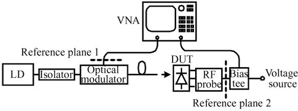
Fig.3 Schematic graph for measurement of  $S_{21}$  (LD: Laser-diode; VNA: Vector network analyzer)
