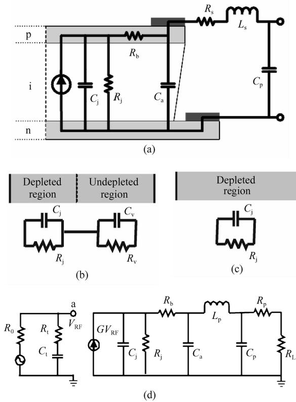
Fig.1 Small-signal equivalent circuit model of a pin photodetector (a) Cross section of a pin-diode; (b) Equivalent circuit of a partly depleted intrinsic region; (c) Equivalent circuit of a completely depleted intrinsic region; (d) Small-signal equivalent circuit model
