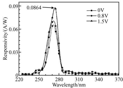
Fig.6 Measured spectral responsivity of the AlGa<sub>N</sub> p-i-n photodetector as a function of reverse bias
