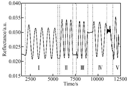
Fig.4 *In-situ* reflectance measurement of the growth process of the AlGaIn p-i-n structure on  $\text{Al}_2\text{O}_3$  substrate
