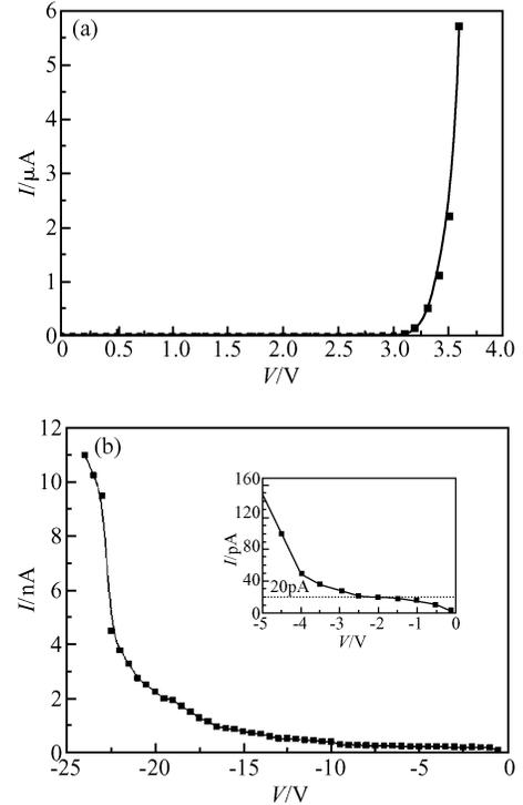
Fig.5  $I$ - $V$  curves for forward bias (a) and reverse bias (b)
