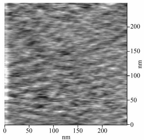
Fig.3 Surface morphology of the AlGa<sub>x</sub>N based p-i-n structure on Al<sub>2</sub>O<sub>3</sub> substrate
