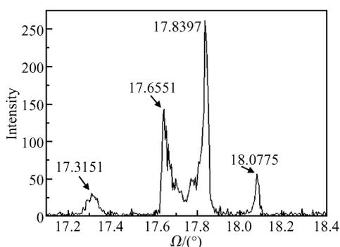
Fig.2 TAXRD curve of the (002) reflection for the detector
