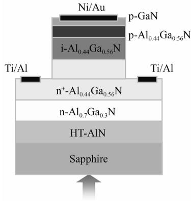
Fig.1 Schematic structure of a back-illuminated p-i-n photodetector
