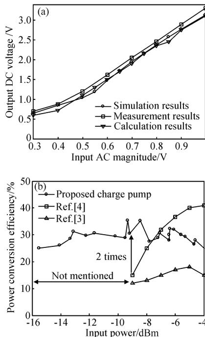
Fig. 11 (a) Calculation, simulation, and measurement results of output voltage with 120kΩ load; (b) Simulation and measurement results of PCE
