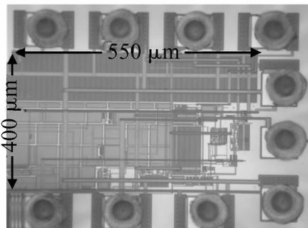
Fig. 10 Micrograph of the proposed analog front-end
