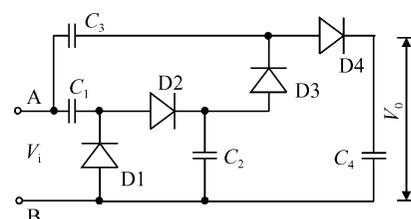
Fig. 3 Conventional charge pump
