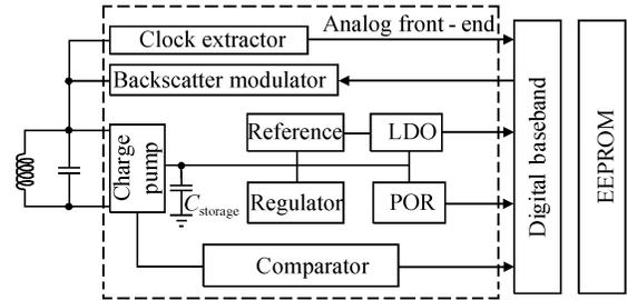
Fig. 2 Architecture of the analog front-end
