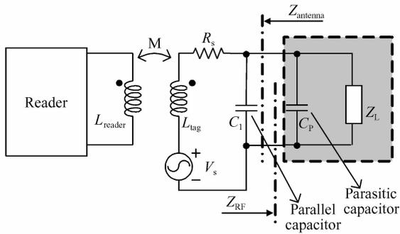
Fig. 1 power transmission in RFID system
