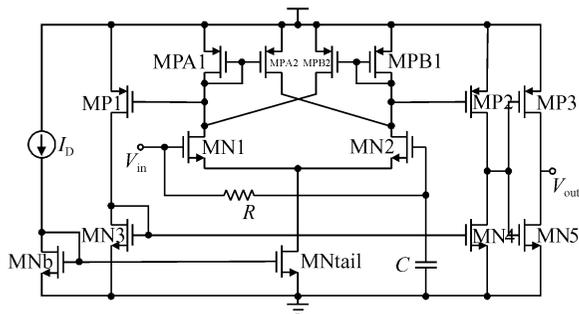
Fig. 8 Comparator schematic
