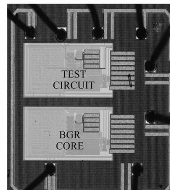
Fig.3 Micrograph of the bandgap reference die
