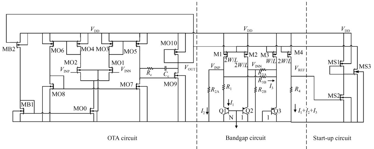
Fig.2 Complete schematic of the proposed low voltage high precision bandgap reference
