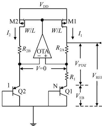
Fig. 1 Conventional CMOS bandgap circuit
