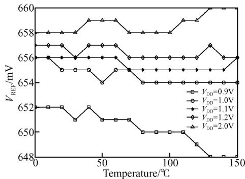
Fig. 5 Measured temperature dependences of the bandgap reference with different  $V_{DD}$
