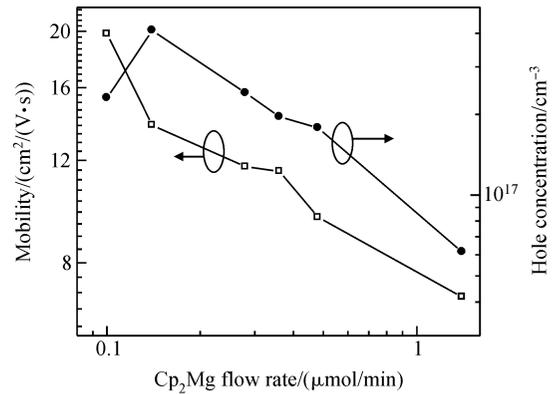
Fig.2 Measured hole concentration and mobility of the six samples with different Mg flow rates
