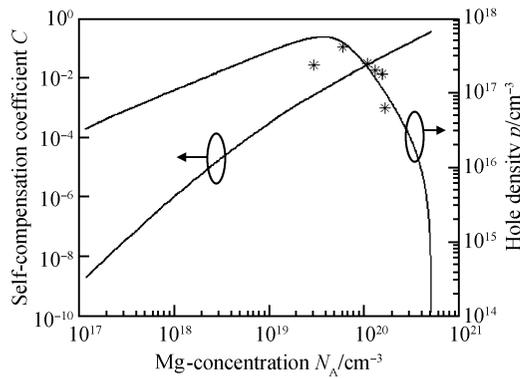
Fig. 3 Calculated hole concentration and self-compensation coefficient as a function of doping concentration
