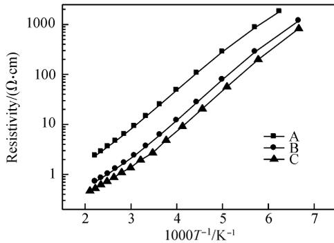
Fig.1 Measured resistivity as a function of temperature on the three Mg-doped GaN samples with different Mg flow rates
