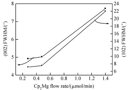
Fig. 4  $Cp_2Mg$  flow rate dependence of FWHM of (002) and (102) faces of the GaN films
