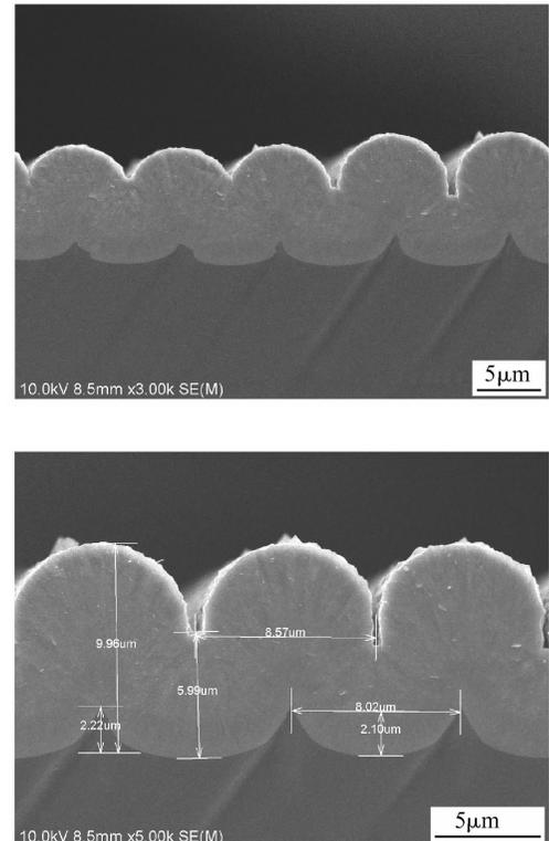
Fig. 2 Cross-sectional SEM micrographs of the 3C-SiC film grown on patterned Si substrate
