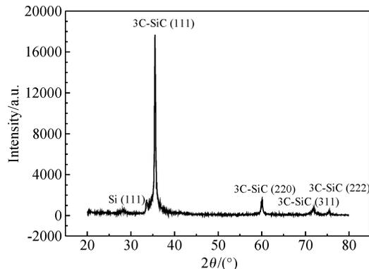
Fig.4 XRD spectrum of the 3C-SiC film grown on patterned Si substrate
