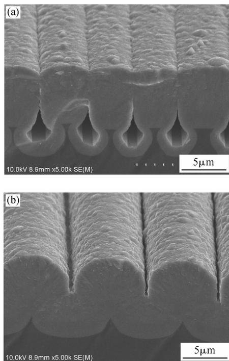
Fig.3 Tilt SEM micrographs of the 3C-SiC films grown on patterned Si substrate (a) Air-gap structure; (b) Spherical shape
