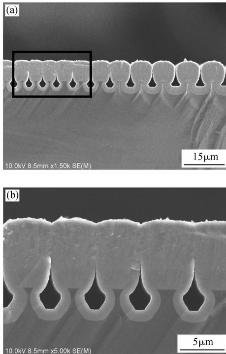
Fig. 1 (a) Cross-sectional SEM micrographs of the 3C-SiC film grown on patterned Si substrate; (b) Magnification of the area marked in (a)
