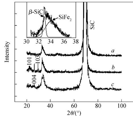
Fig.3 XRD spectra of the prepared sample corresponding to different annealing stages of the HNH process (a) Annealing in hydrogen atmosphere at 300°C for 5min; (b) Based on (a), annealing in nitrogen atmosphere at 700°C for 5min; (c) Based on (b), annealing in hydrogen again at 250°C for 5min
