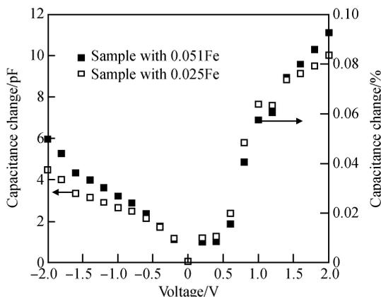
Fig. 6 Curves of capacitance-voltage corresponding to different Fe concentrations
