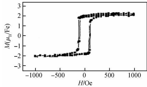
Fig. 7 Hysteresis loops of  $\text{Si}_{0.95}\text{Fe}_{0.05}\text{C}$  in different orientations with respect to the applied field at  $T = 200\text{K}$
