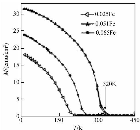
Fig.4 Magnetization as a function of temperature in a 50Oe field for several different Fe concentrations
