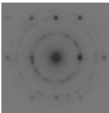
Fig.2 Selective area electron diffraction pattern (SADP) of the 4H-SiC:Fe DMS sample
