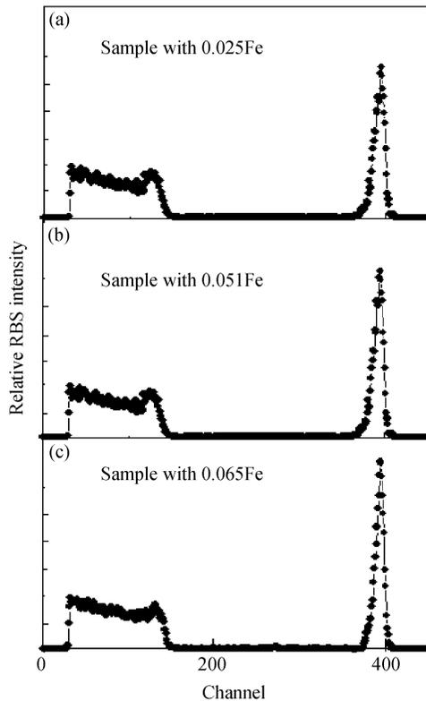
Fig. 5 RBS spectra for samples with different Fe concentrations
