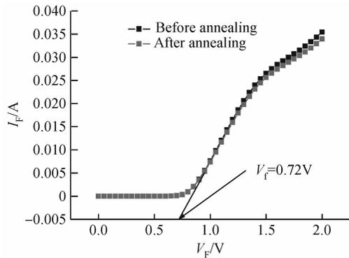
Fig. 5  $I$ - $V$  characteristic curve of gate Schottky barrier diode
