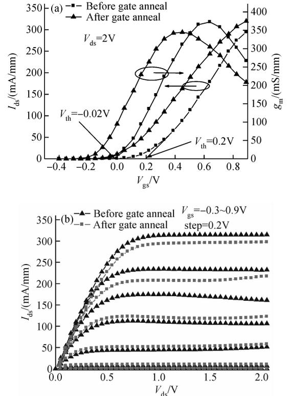
Fig. 3 Transfer characteristics & DC characteristics of  $1 \mu\text{m}$  E-PHEMT with Ti/Pt/Au gate (before and after gate anneal)
