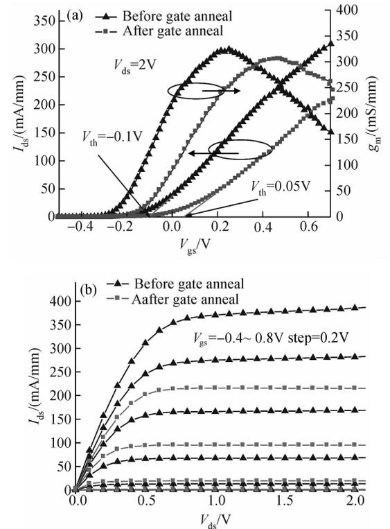
Fig. 4 Transfer characteristics & DC characteristics of  $1 \mu\text{m}$  E-PHEMT with Pt/Ti/Pt/Au gate (before and after gate anneal)
