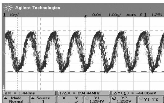
Fig. 6 Nine-stages ring oscillator
