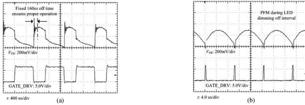
Fig.8. Feedback and gate drive signal in (a) CCM and (b) DCM operation.
