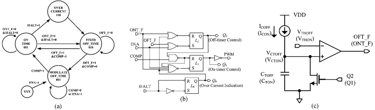
Fig.3. COT logic: (a) COT state-chart; (b) Synthesized of the control FSM; (c) Simplified circuit scheme of the off timer.
