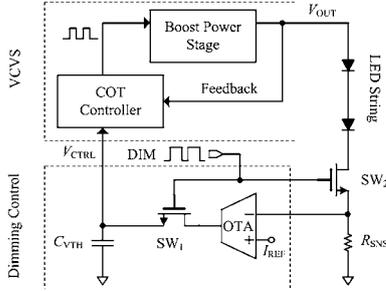
Fig.1. Block diagram of the proposed LED drive system.
