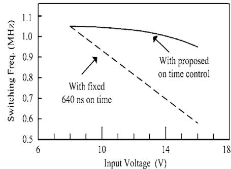
Fig.10. Operation frequency variation comparison with and without the on time control.
