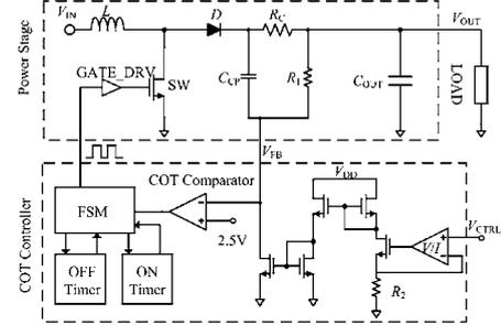
Fig.2. Schematic of the COT boost converter.
