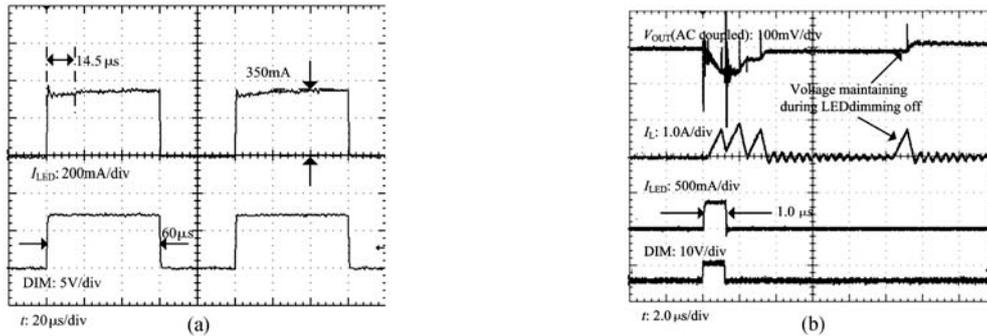
Fig.9. LED lamp dimming test: (a) Long dimming on time test; (b) Minimum dimming on time test.
