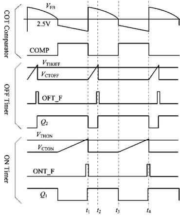
Fig.4. Key waveforms of the COT logic in CCM.
