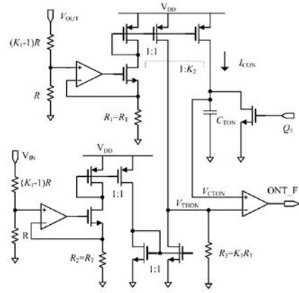
Fig.5. Proposed on time generator for CCM frequency control.
