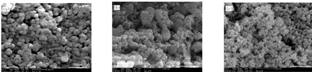
Fig. 1. Characterization of materials sintered at 600 °C by SEM: (a) In-Nb; (b) In-Cd; (c) In-Mg.
