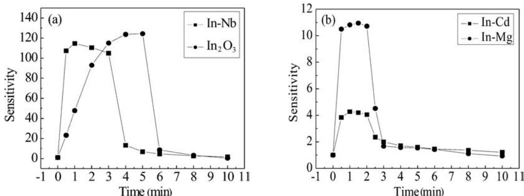
Fig. 2. Response and recovery characteristic curves: (a) In-Nb and In<sub>2</sub>O<sub>3</sub>; (b) In-Cd and In-Mg.
