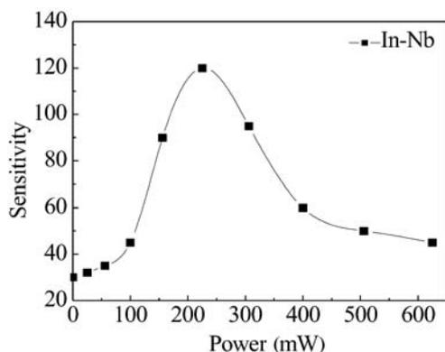
Fig. 4. Relationship between heating power and sensitivity.
