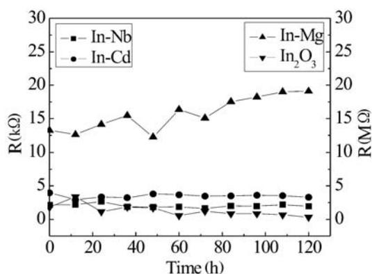
Fig. 3. Thermal stability of different doping materials during 120 h.
