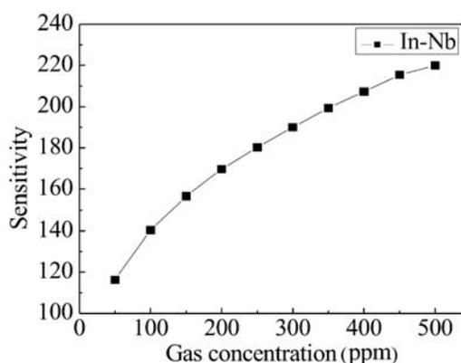
Fig. 5. Relationship of gas concentration and sensitivity.
