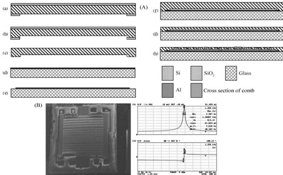
Fig. 6. (A) Fabrication process flow of the device; (B) Device testing grid strip capacitance and tested Q curves.
