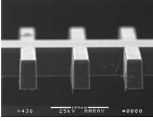
Fig. 4. SEM picture of the cross section of non-parallel combs.
