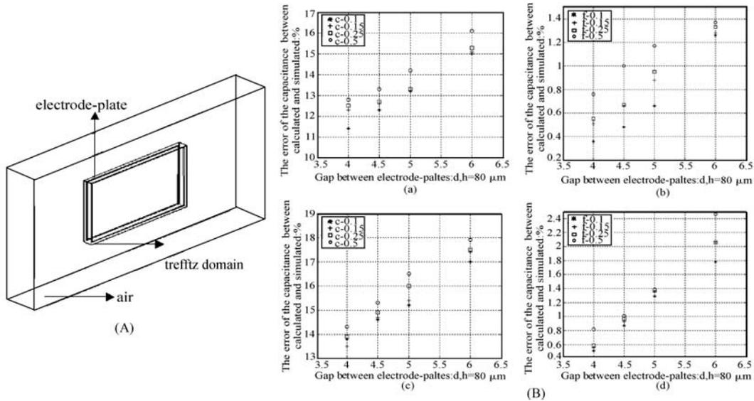
1. Trefftz domain of the oblique combs 2. Error of simulated and computed results of capacitance and electrostatic force
