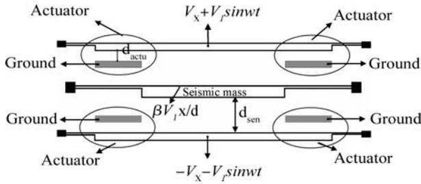
Fig. 1. The simplified schematic structure of the accelerometer.
