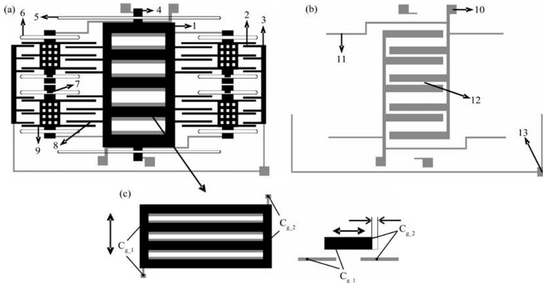
1. seismic mass 2. driving capacitor of the actuator 3. supporting anchor of the actuator 4. supporting anchor of the accelerometer 5. U-shape sensitive beam 6. beam of the actuator 7. pull-in heave 8. sensing capacitor 9. actuator 10. bonding of the sensitive mass 11. connecting line between capacitors 12. grid strip aluminum electrodes 13. bonding of the actuators.
