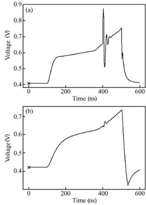
Fig. 5. Simulation result of anti-jamming performance: (a) Traditional current-sensing circuit; (b) Proposed current-sensing circuit.
