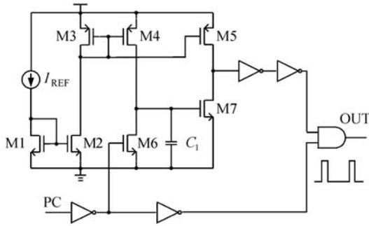
Fig. 3. Schematic of one-shot circuit.
