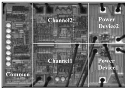
Fig. 6. Micrograph of the achieved DC-DC converter.
