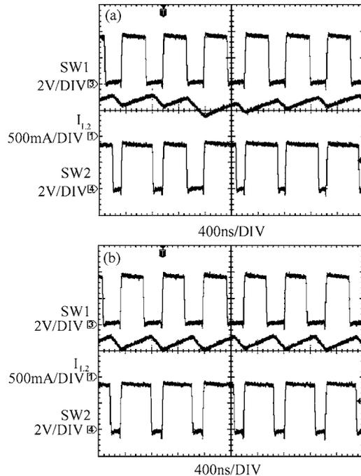
Fig. 7. Measured waveforms of  $I_L$  and SWs: (a) With traditional current-sensing circuit; (b) With proposed current-sensing circuit.  $V_{IN} = 3.6$  V,  $V_{OUT1} = 1.8$  V,  $V_{OUT2} = 2.4$  V,  $I_{LOAD1} = I_{LOAD2} = 600$  mA.
