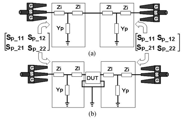
Fig. 2. Test structures: (a) The 'Through' dummy; (b) DUT with the pads.
