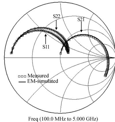
Fig. 8. Comparison between measured and EM-simulated  $S$ -parameters.
