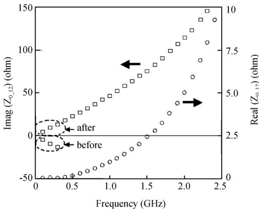
Fig. 6. Calculated coupling impedance  $Z_{0,12}$  before and after the data correction.
