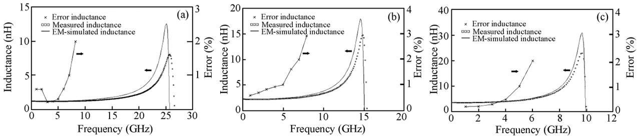
Fig. 4. Comparison between measured and EM-simulated inductances: (a) R40T3; (b) R40T4; (c) R40T5.
