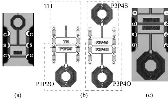
Fig. 1. (a) Die photo of R60T3.654; (b) Test structures of a transformer; (c) Die photo of P3P4O.
