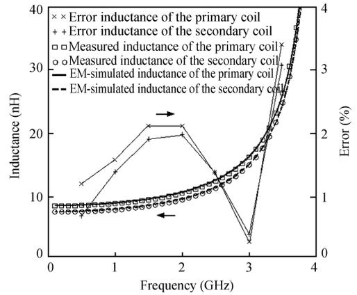
Fig. 7. Comparison between measured and EM-simulated coil inductances.
