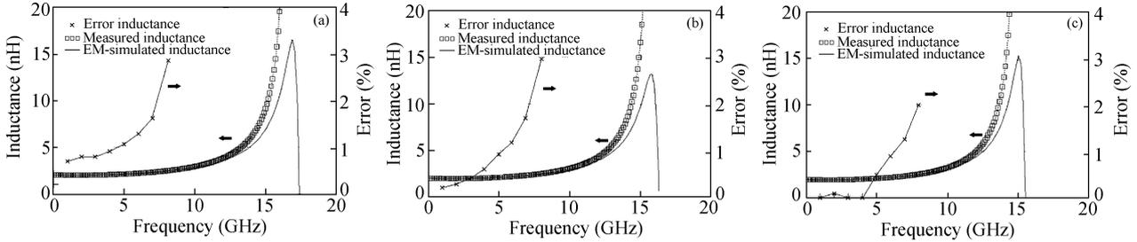
Fig. 5. Comparison between measured and EM-simulated inductances: (a) R60T3.6; (b) R60T3.65; (c) R60T3.654.
