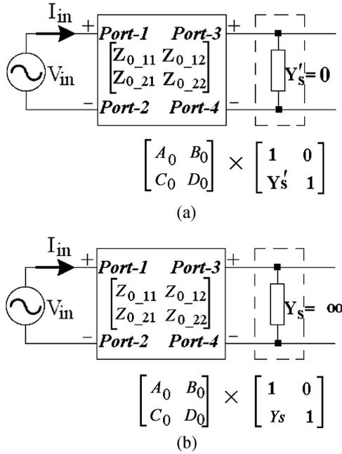
Fig. 3. Definition of  $Z_{11}$  in differentially-excited modes of (a) P3P4O and (b) P3P4S.
