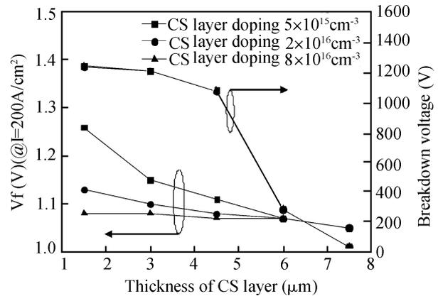
Fig. 8. Characteristics of PF-CSTBT with different thicknesses of CS layers when  $X_j = 1.2 \mu\text{m}$ .
