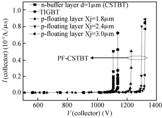
Fig. 5. Breakdown voltage of CSTBT, TIGBT and PF-CSTBT with different p-floating layers.
