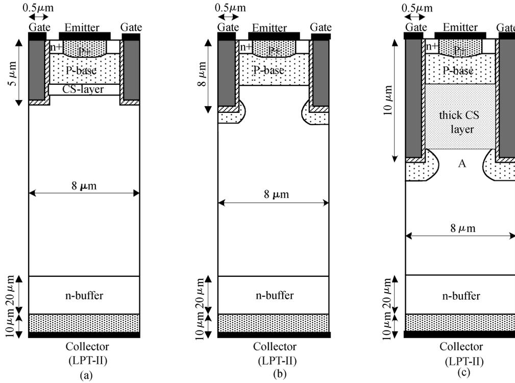
Fig. 1. (a) CSTBT. (b) P-FIGBT. (c) PF-CSTBT.
