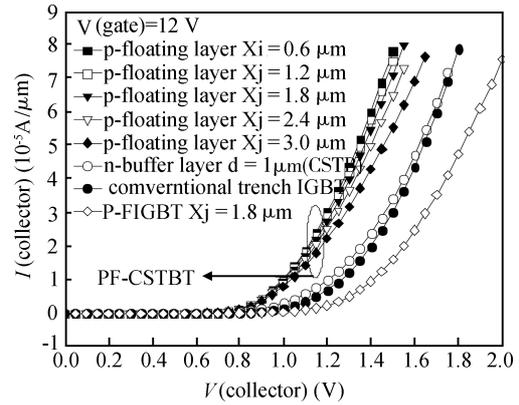
Fig. 3. Comparison between  $I-V$  characteristics of different p-floating layers.
