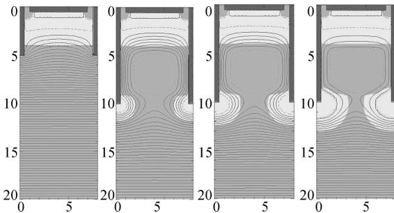
Fig. 6. Potential distribution of (a) conventional IGBT and various p-floating layers of PF-CSTBT [(b)  $X_j = 0.6 \mu\text{m}$ , (c)  $X_j = 1.8 \mu\text{m}$ , (d)  $X_j = 3.0 \mu\text{m}$ ].
