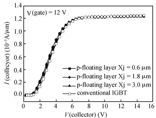
Fig. 4. Comparison of saturation current.
