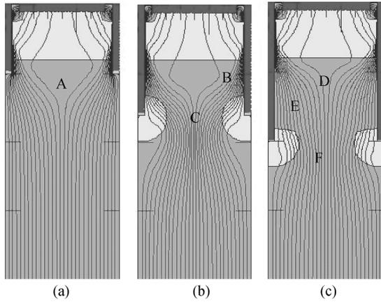
Fig. 2. Current distribution of (a) conventional IGBT, (b) P-FIGBT, and (c) PF-CSTBT at  $V_{gate} = 12\text{ V}$ ,  $V_{collector} = 8\text{ V}$ .
