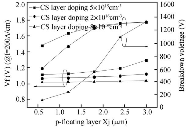
Fig. 7. Characteristics of PF-CSTBT with various p-floating areas and CS layer concentrations.
