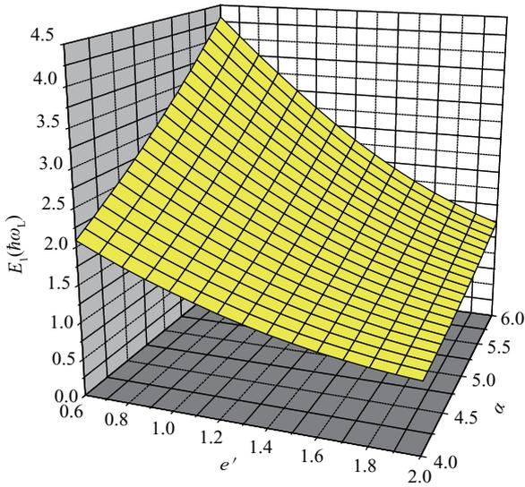
Fig. 1. Relational curves of the first internal excited state energy  $E_1$  with the electron–phonon coupling strength  $\alpha$  and the aspect ratio  $e'$  of the ellipsoid for fixed  $l_p = 4$  and  $l_v = 2$ .
