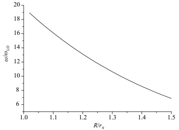
Fig. 4. Relational curves of the frequency  $\omega$  of the transition spectral line with the transverse radius  $R$  of quantum rods for fixed  $l_p = 2$ ,  $l_v = 3$ ,  $L = 5.5$  and  $\alpha = 4$ .
