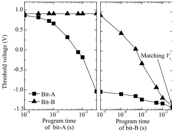
Fig. 6. Restrain on the interference between bit-A and bit-B during program operation.
