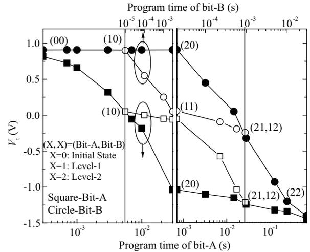
Fig. 9. 3-bit/cell storage characteristic of NUC-CTM and the program speed of each bit.
