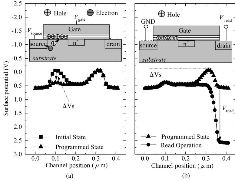
Fig. 3. (a) Source-side program and (b) source-side read operation principle of the NUC-CTM cell.
