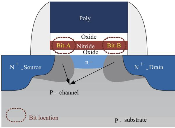
Fig. 1. Structure of a single NUC-CTM cell.
