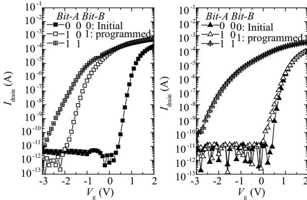
Fig. 7.  $I_{\text{drain}}/I_{\text{source}}-V_g$  curve of the NUC-CTM with different states of bit-A and bit-B.
