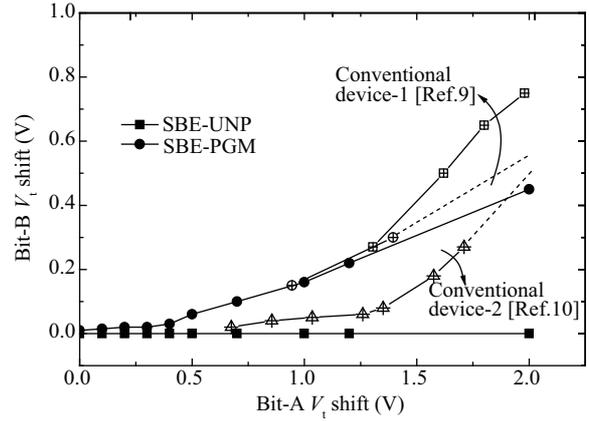
Fig. 8. SBE-UNP and SBE-PGM induced  $V_t$  shifts in the NUC-CTM and other mirror-bit storage devices<sup>[9, 10]</sup>.
