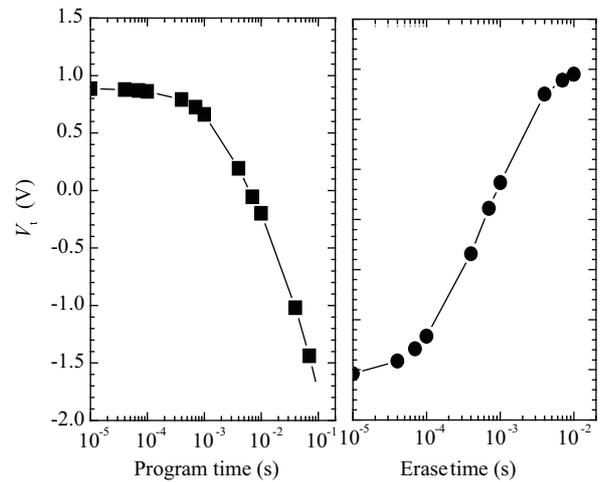
Fig. 5. Program/erase characteristic of the NUC-CTM cell.
