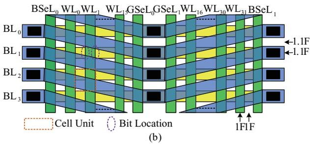
Fig. 4. (a) Schematic diagram of the proposed virtual-source NAND type array structure. (b) Top view layout of the proposed VS-NAND structure.
