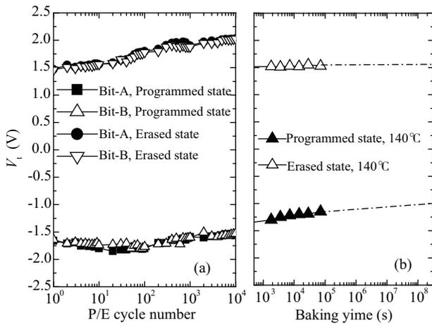
Fig. 10. (a) Endurance and (b) retention characteristic of the NUC-CTM.
