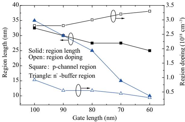
Fig. 2. Simulation results of scalability of NUC-CTM. The gate length can scale down below 60 nm by carefully controlling the length and doping of the p-channel region and the  $n^-$ -type buffer region.
