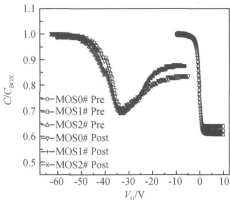
Fig. 3 High frequency  $C-V$  characteristics of MOS 0# ~ 2 # capacitors measured at a frequency of 1MHz before and after  $5 \times 10^5$  rad (Si) irradiation Gate bias is 0V during irradiation.
