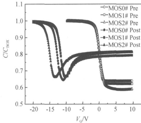
Fig. 2 High frequency  $C-V$  characteristics of MOS 0# ,2# capacitors measured at a frequency of 1MHz before and after  $1 \times 10^5$  rad (Si) irradiation Gate bias is 6.5V during irradiation.
