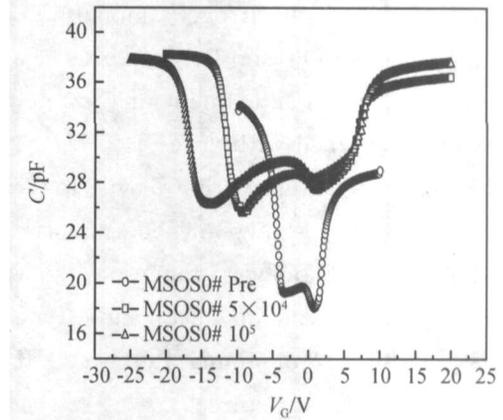
Fig. 4 High frequency  $C-V$  characteristics of MSOS 0# capacitor measured at 1MHz before and after  $5 \times 10^4$  and  $10^5$  rad (Si) irradiation. Gate bias is 6.5V during irradiation.
