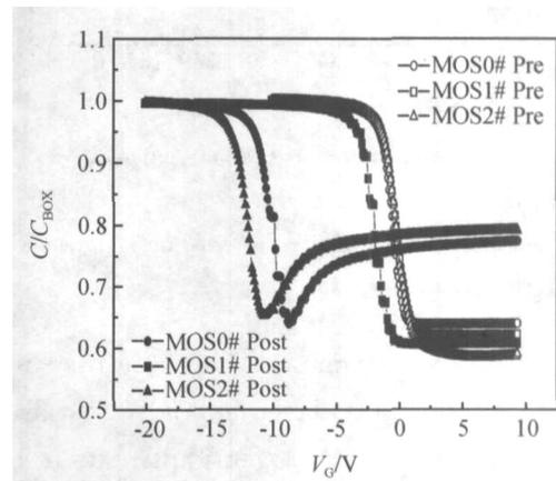
Fig. 1 High frequency  $C-V$  characteristics of MOS 0# ~ 2# capacitors measured at a frequency of 1MHz before and after  $5 \times 10^4 \text{rad(Si)}$  irradiation Gate bias is 6.5V during irradiation.
