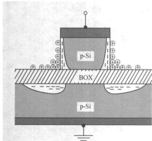
Fig. 5 Schematic illustration of permanent inversion layers caused by positive impurity ions for a MSOS structure before irradiation
