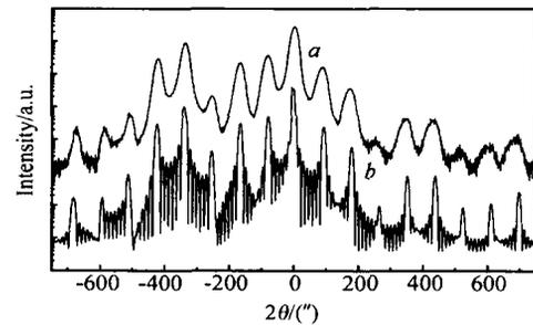
Fig. 1 DCXRD rocking curves of the as-grown  $\text{Al}_x\text{Ga}_{1-x}\text{As}/\text{GaAs}$  DBR. Curve *a*: the measured curve; Curve *b*: the simulated curve
