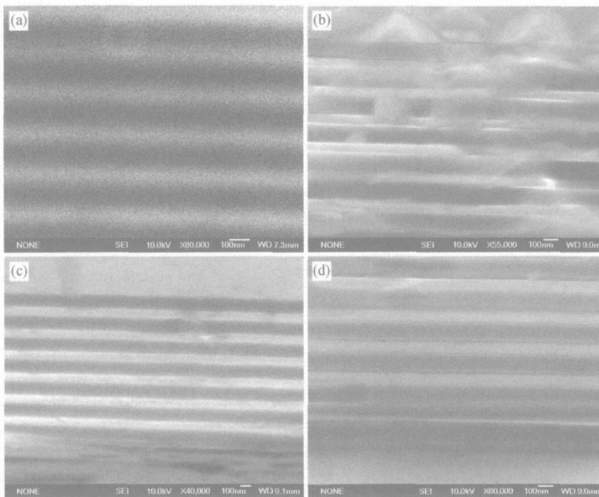
Fig. 3 Cross-sectional SEM images of DBR (a) As-grown; (b) Oxidized for 12min; (c) Oxidized for 20min; (d) Oxidized for 40min
