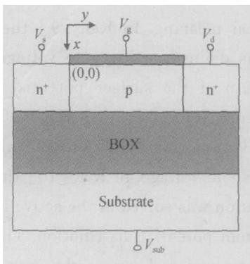
Fig.1 Cross-section of an n-channel SOI MOSFET
