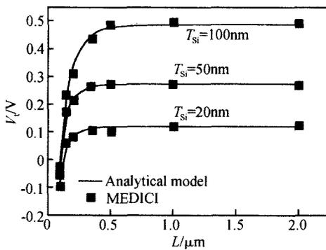
Fig. 4 Threshold voltage versus gate length for different silicon film thicknesses. The devices parameters are:  $T_{\text{tox}} = 10\text{nm}$ ,  $T_{\text{box}} = 320\text{nm}$ ,  $N_{\text{ch}} = 1.2 \times 10^{17}\text{cm}^{-3}$ ,  $V_{\text{ds}} = 0.05\text{V}$ .
