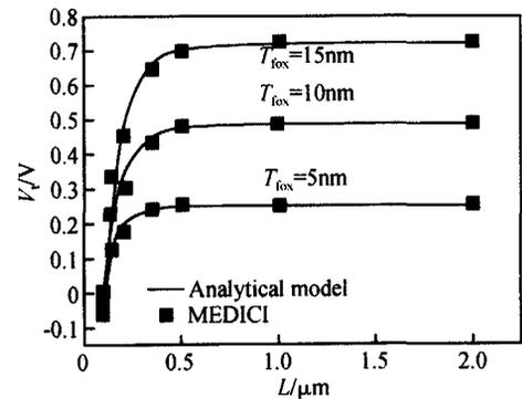
Fig. 3 Threshold voltage versus gate length for different gate oxide thicknesses. The device parameters are:  $T_{Si} = 100\text{nm}$ ,  $T_{box} = 320\text{nm}$ ,  $N_{ch} = 1.2 \times 10^{17}\text{cm}^{-3}$ ,  $V_{ds} = 0.05\text{V}$ .
