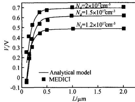
Fig. 5 Threshold voltage versus gate length for different channel doping concentrations. The devices parameters are:  $T_{\text{tox}} = 10\text{nm}$ ,  $T_{\text{box}} = 320\text{nm}$ ,  $T_{\text{Si}} = 100\text{nm}$ ,  $V_{\text{ds}} = 0.05\text{V}$ .
