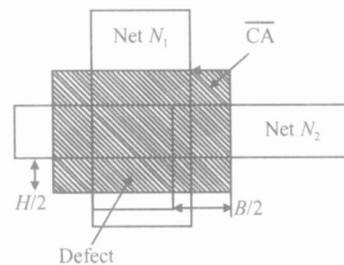
Fig. 3 Critical area of net pairs  $(N_1, N_2)$  of adjacent layers  $I, J$
