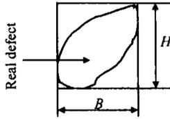
Fig. 1 Rectangular model of a real defect  $D(H, B)$
