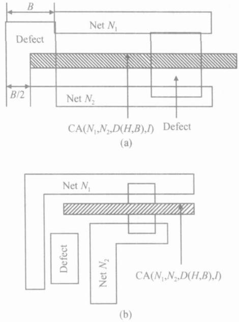
Fig. 2 (a) Critical area of the horizontal net pairs  $(N_1, N_2)$  ;(b) Critical area of net pairs  $(N_1, N_2)$
