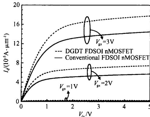
Fig. 7 Simulated output characteristics of the DGDT and conventional FDSOI nMOSFET
