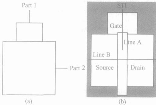
Fig. 1 (a) Layout of the active island composed of Part 1 and Part 2. Part 1 and the BOX layer below it will be partially etched off for the connection between the front-gate polysilicon and back-gate n-well; (b) Layout of the nMOSFET
