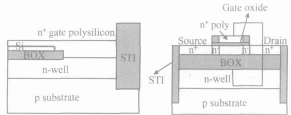
Fig. 2 (a) Cross section along line A showing the contact between the front-gate and back-gate n-well; (b) Schematic cross section of the device along line B
