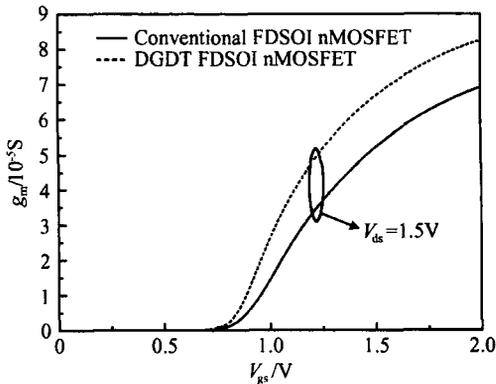
Fig. 9 Simulated transconductance characteristics of the DGDT and conventional FDSOI nMOSFETs with the drain biased at 1.5V
