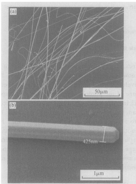
Fig. 1 SEM images of typical as-grown ZnO nanowires (a) Overhead view of ZnO nanowires; (b) Close-up of a 425nm-diameter
