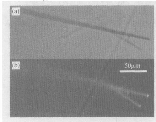
Fig. 6 Photoluminescence observed in a ZnO nanowire when it is excited at 325nm by means of evanescent coupling (a) Before excitation; (b) After excitation
