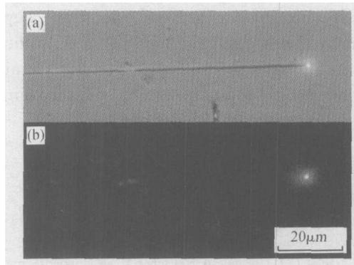
Fig. 5 Optical micrograph of a ZnO nanowire guiding 633nm light on the surface of a silicate glass substrate (a) With external illumination; (b) Without external illumination
