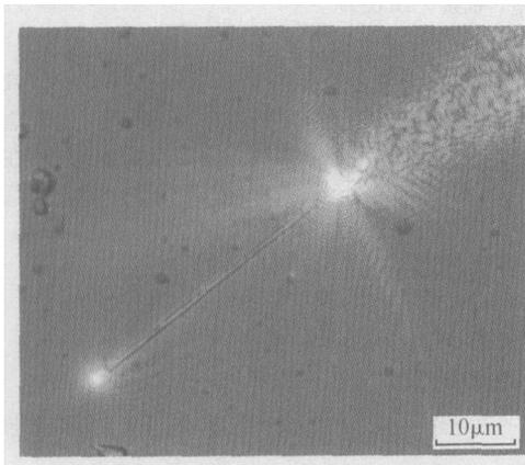
Fig. 4 Optical micrograph of launching 633nm light into a ZnO nanowire by means of a silica nanotaper
