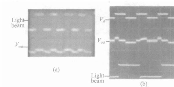
Fig. 5 Input and output waveforms of optoelectric integrated circuit (a) Opto-controlled switch; (b) Opto-controlled inverter
