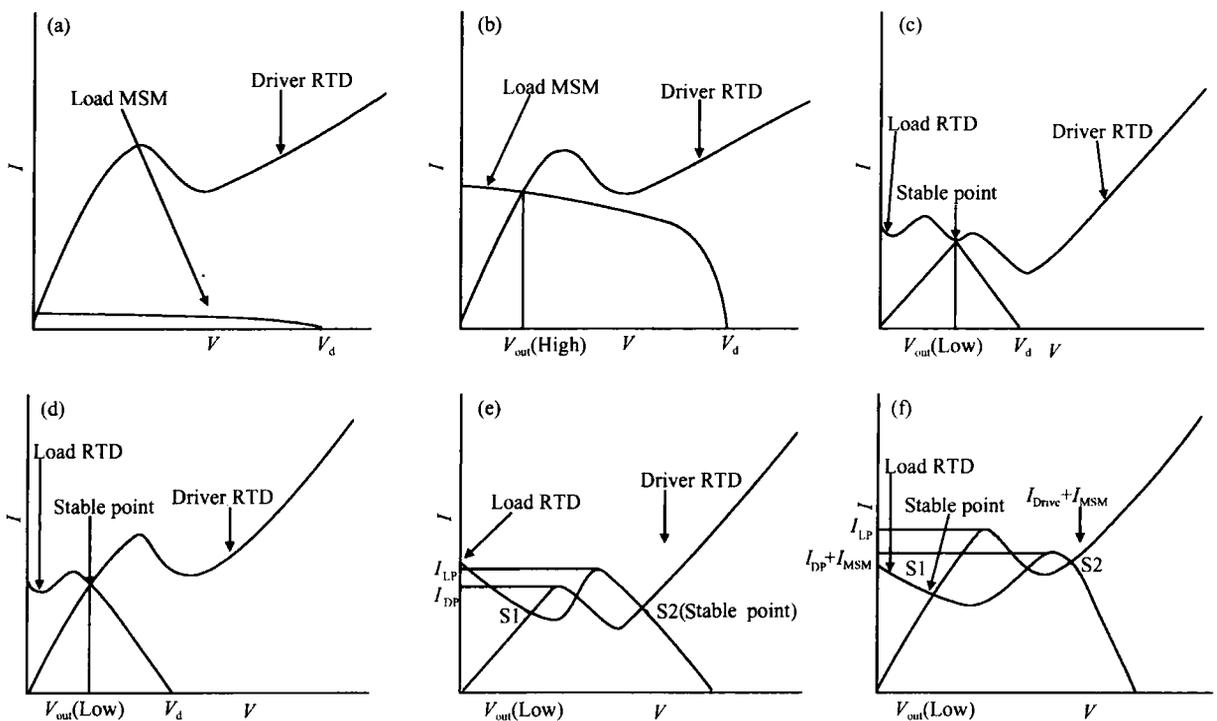
Fig. 2 Operation principle of OEIC (a) Un-illuminated (switch); (b) Illuminated (switch); (c) Un-illuminated and low-level clock (inverter); (d) Illuminated and low-level clock (inverter); (e) Un-illuminated and high-level clock (inverter); (f) Illuminated and high-level clock (inverter)
