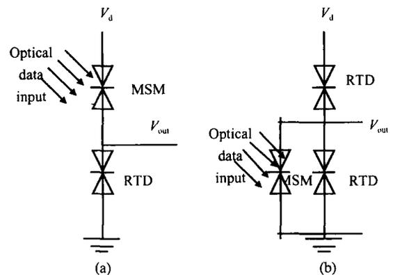
Fig. 1 Circuit diagram of monolithic opto-controlled negative difference solid circuits
