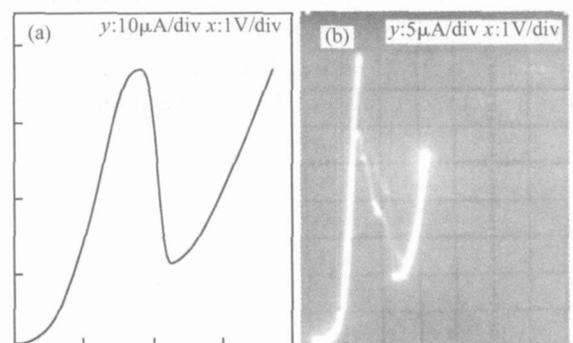
Fig. 4 (a) Simulated *FV* curve of the RTD by PSPICE; (b) Measured *FV* curve of the RTD
