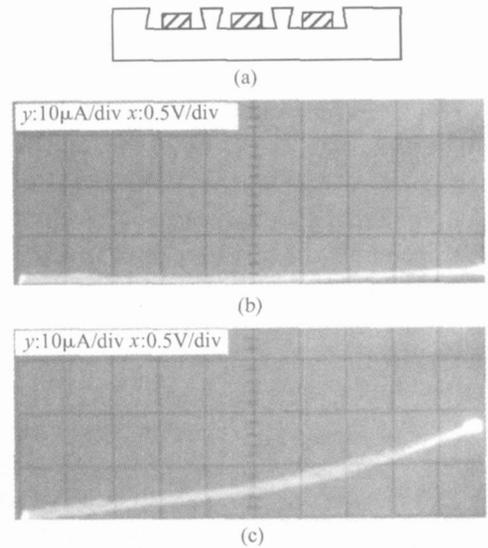
Fig. 3 (a) Schematic cross section of MSM; (b) *FV* curves of MSM without the swallow trench; (c) *FV* curves of MSM with the recessed electrodes
