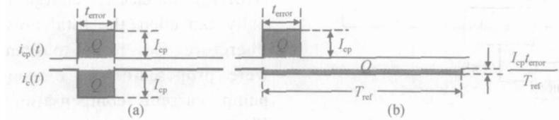
Fig. 5 (a) Compensation current exactly cancels the noisy electric charge ;(b) Compensation current injected during the whole reference period
