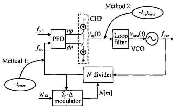
Fig.2 Structure of the sigma-delta fractional-N frequency synthesizer
