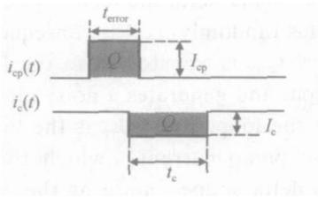
Fig. 4 Illustration of charge pump current compensation to the sigma-delta induced noise
