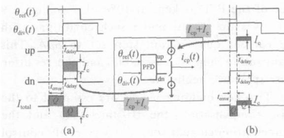
Fig. 6 Proposed compensation scheme (a)  $f_{ref}$  leads to  $f_{div}$ ; (b)  $f_{div}$  leads to  $f_{ref}$
