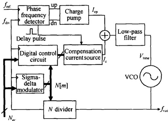
Fig. 7 Functional block diagram of the proposed synthesizer
