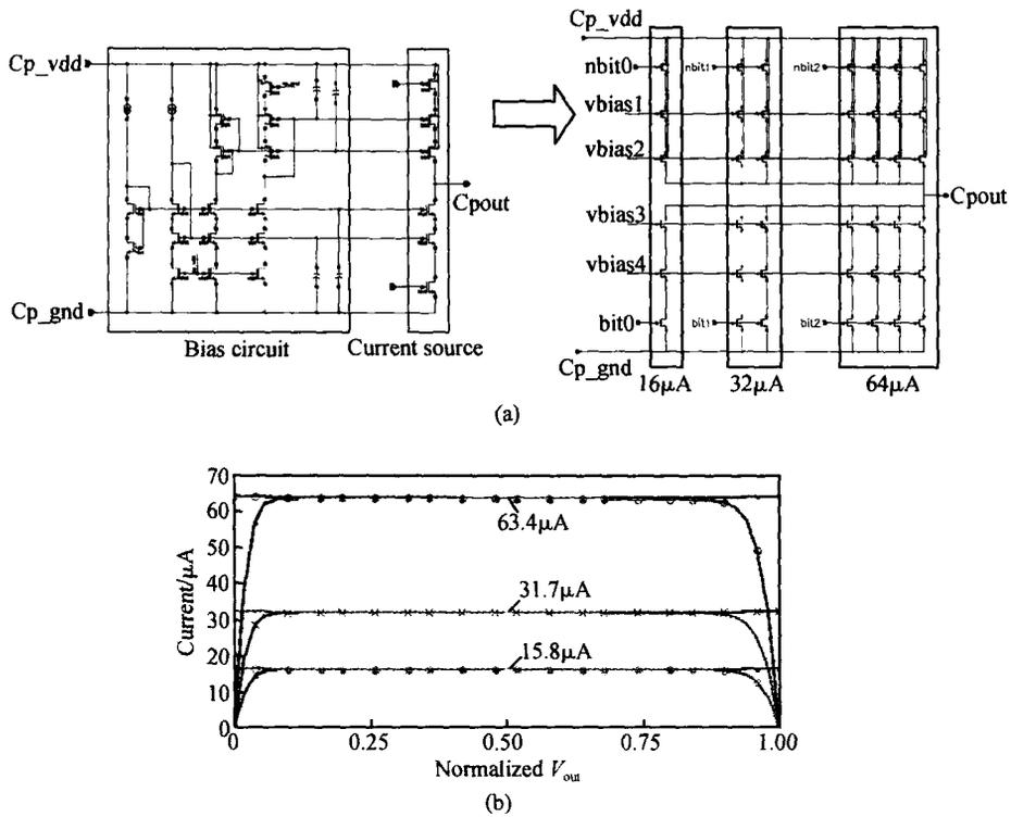
Fig. 11 (a) Binary-weight compensation current source ;(b) Simulation results of the compensation current
