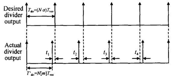
Fig. 3 Ideal and actual frequency divider output signal in the time domain
