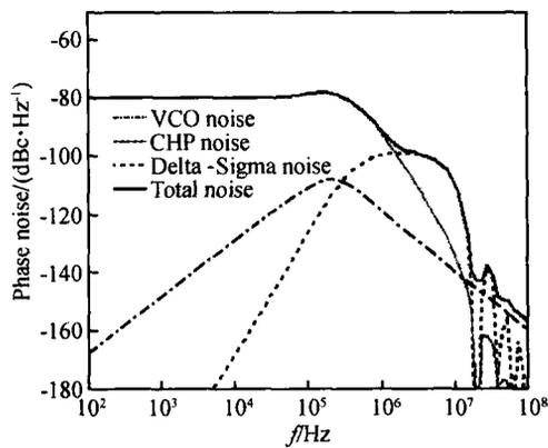
Fig.1 Behavior simulation results of the phase noise for a sigma-delta fractional-N frequency synthesizer with a bandwidth of 300k Hz
