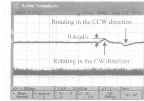
Fig. 5 Upper curve is the gyro signal from LIA1 when the R-FOG is rotating while the lower curve is the output signal from PD2.
