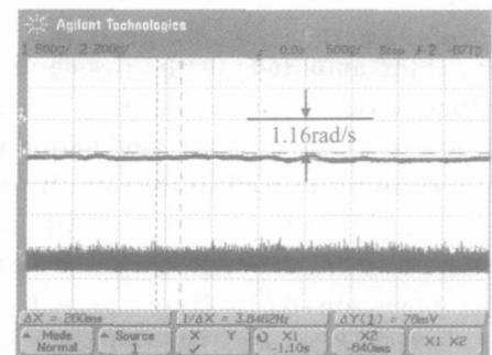
Fig. 6 Upper curve is the gyro signal from LIA1 when the R-FOG is at rest and the lower curve is the output signal from PD2.
