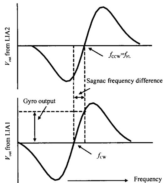
Fig. 3 Diagram of the gyro output signal The R-FOG rotates in the CW direction.
