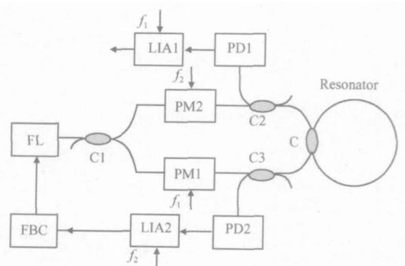
Fig. 1 Diagram of R-FOG using PM spectroscopy
