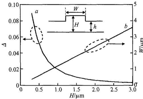
Fig.1 Dependence of refractive index difference ( $\Delta$ ) and waveguide width ( $W$ ) on substrate thickness ( $H$ ) for  $h/H = 2/3$
