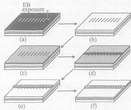
Fig.2 Fabrication process of Bragg gratings on rib waveguides
