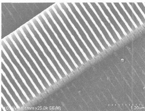
Fig. 3 Bragg grating on an SOI rib waveguide
